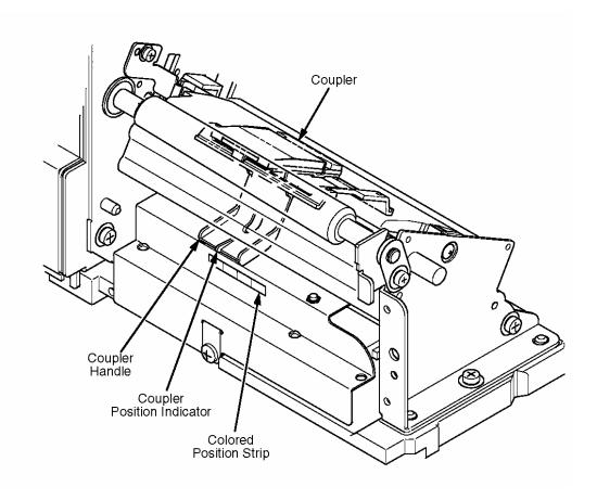
Use the coupler handle to adjust the coupler so that the coupler position indicator points to the correct color on the colored position strip.
